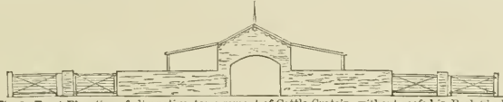
Fig. 3. Front Elevation of alternative Arrangement of Cattle Curtain, without roofed-in Back Sheds.
