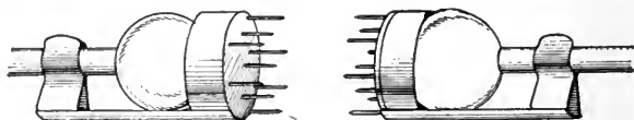
These Shunt Terminals Permit the Giving of Positive Spray with Little Danger of Spark.
