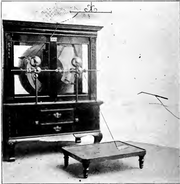
Grounding the Static Machine by Wire Attached to Upper Part of Case, Which Can Easily be Transferred to Opposite Pole.
