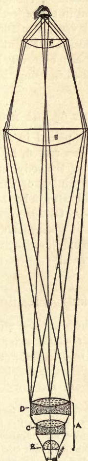
FIG. 2.—DIAGRAM SHOWING THE RELATION OF THE OBJECTIVE TO THE EYE-PIECE.
