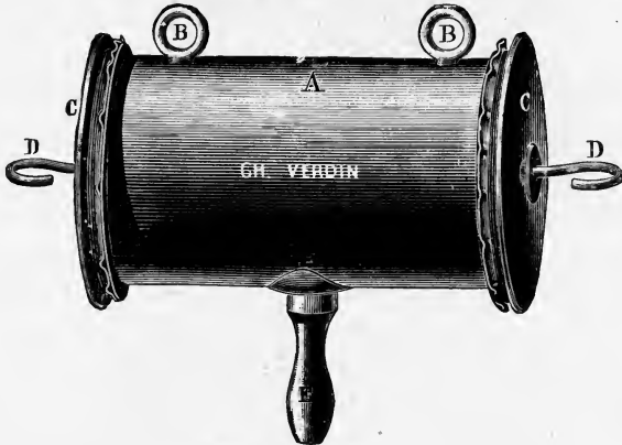
FIG. 117.—Stethograph. A, Metal drum; B, hooks for tapes which pass round neck; C, rubber discs; D, hooks for attaching tapes which are tied round thorax; E, tube leading to the recording tambour.
