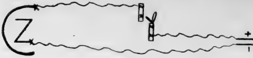
FIG. 82.—Plan of the use of a Du Bois key, as a simple make and break key.
