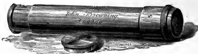
FIG. 179.—Small direct vision spectroscope.
