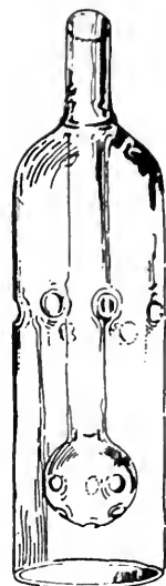
FOLIN IMPROVED ABSORPTION TUBE.
