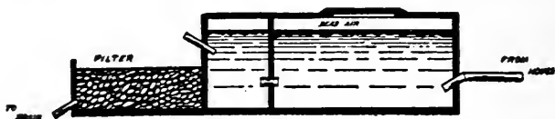
Fig. 18.—The septic tank
