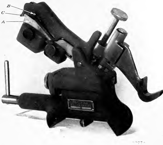
Automatic Positive Feeding Back-rests for Cylindrical Grinders
