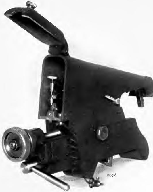
Automatic Sizing Device: 4 x 30 and 6 x 48-inch Cylindrical Grinders
