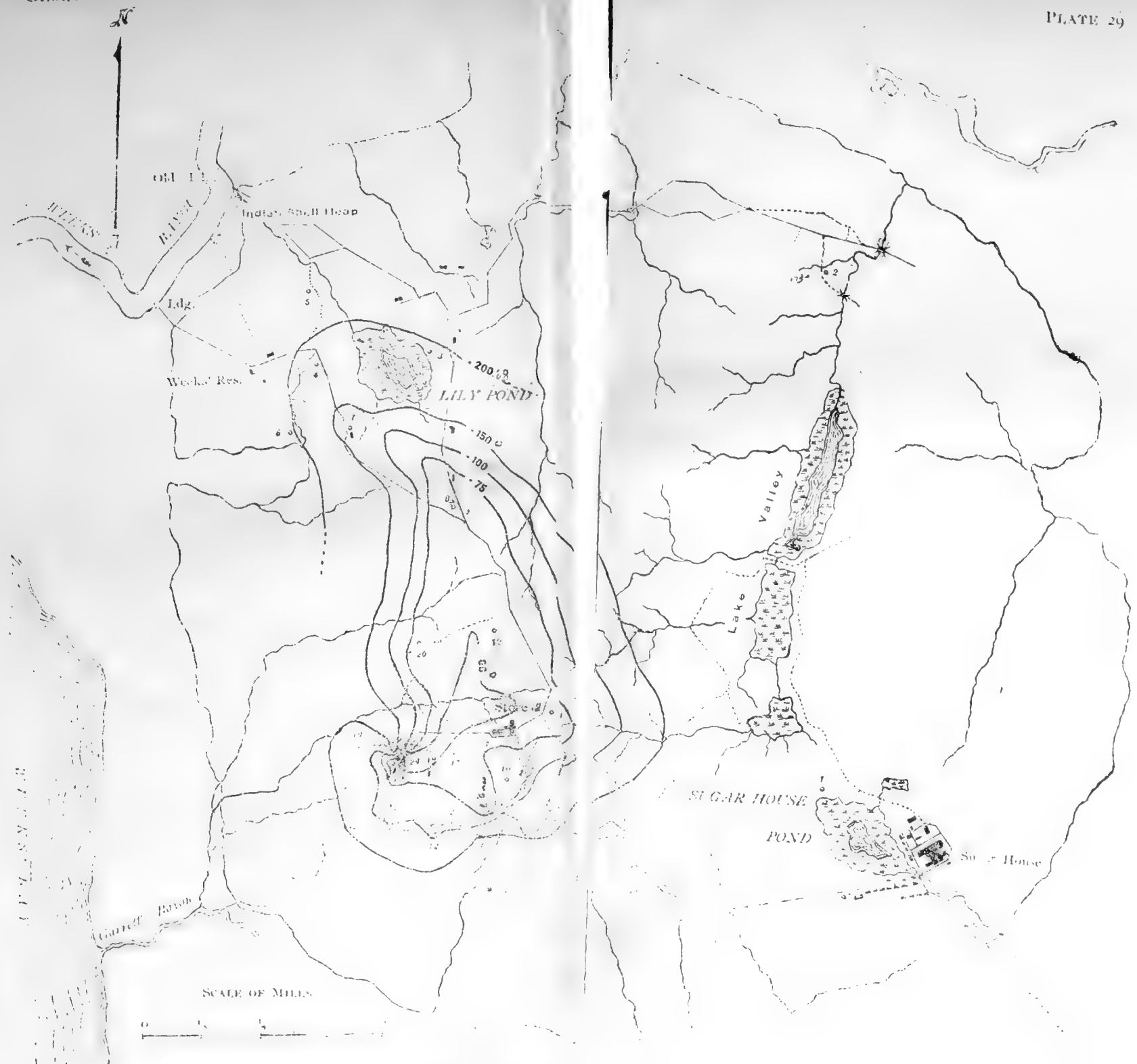
Contour Map of the Salt Deposit of Grande Cote. Elevation given in feet below Gulf Level BY A. C. VEATCH
