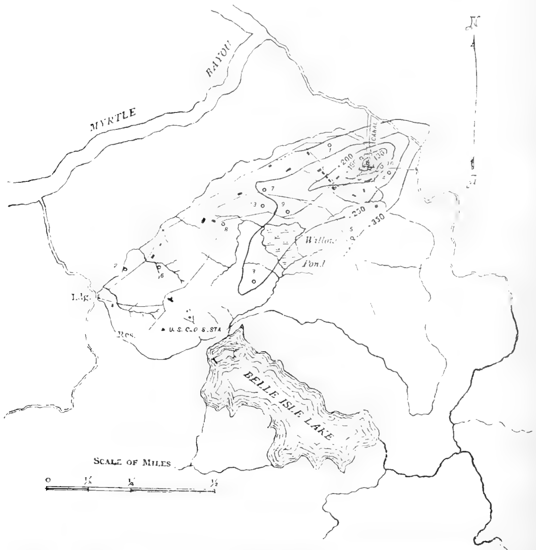
Contour Map of the Salt Deposit on Belle Isle. Elevation given in feet below Gulf Level
