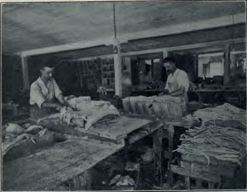
FIG. 2.—Cutting fish for tablets or fish cakes. (The miter box is used by one cutter and the slitted table top by the other.)
