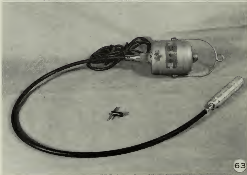
Figure 63 Electric drill with flexible shaft and grinder.
