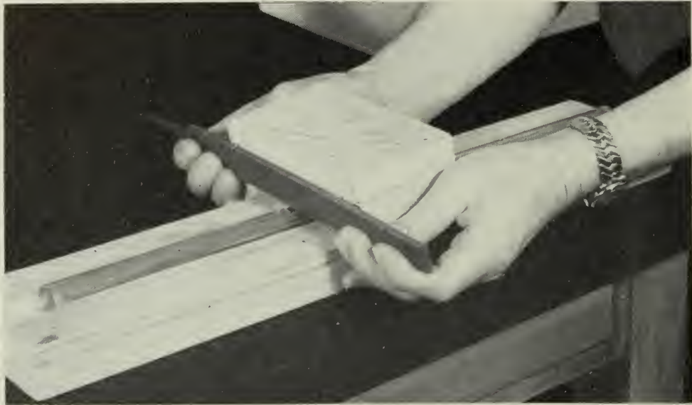
Figure 38—Tool for scribing striæ on enlarged plastic models of wheat stems.
