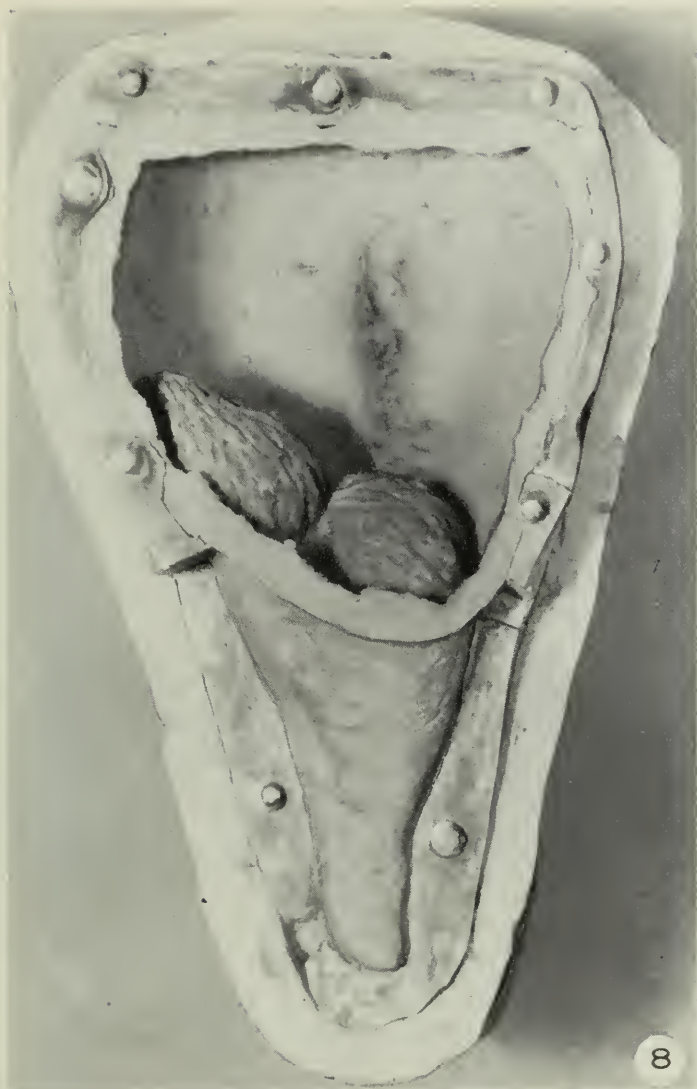
Figure 8 —Rubber mold in plaster jacket showing treatment of undercuts in a sugar beet.
