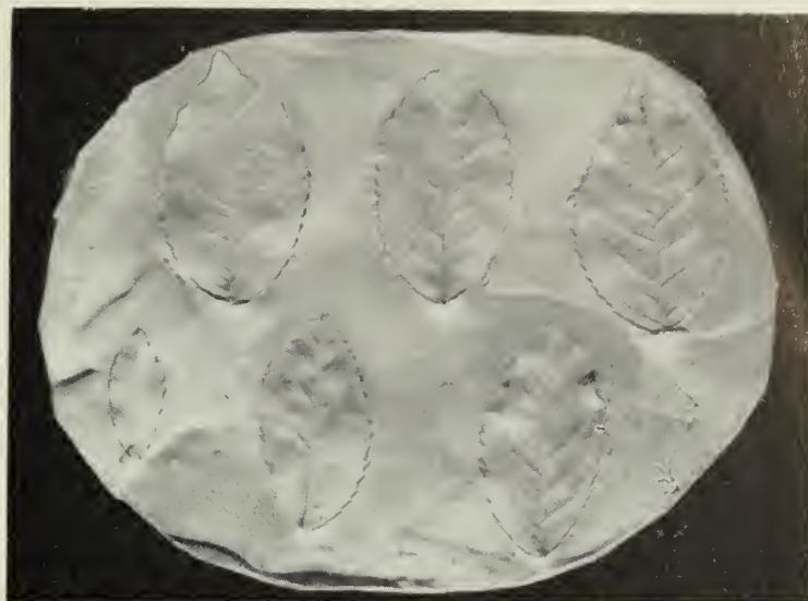
Figure 32 Rubber mold for casting leaves in liquid plastic.
