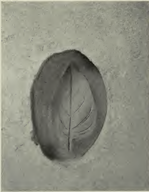
Figure 16 Impression in molders' sand from mold on leaf.
