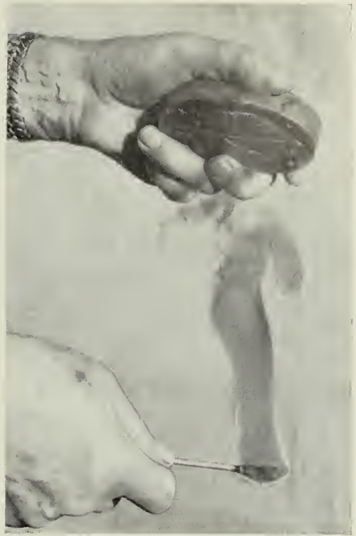
Figure 18 —Metal mold is smoked to form a separator for the second pour.
