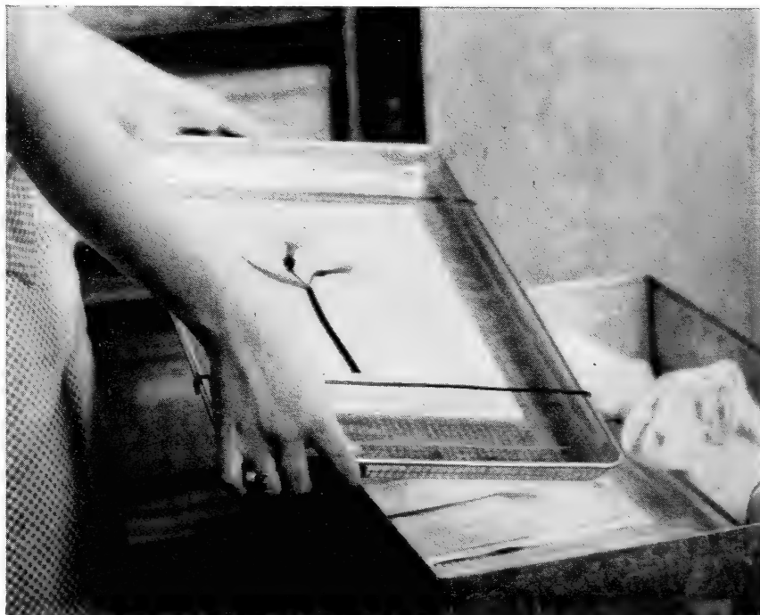
FIGURE 5.—Preserved specimens laid out on plastic sheets under temporary cover films of cellulose acetate are dehydrated in a tightly closed box containing a suitable desiccant.
