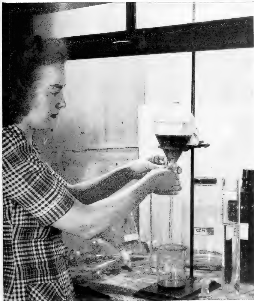
FIGURE 11.—A separatory funnel is used when removing inhibitor by the alkali-extraction method. The operation should be carried out under a fume hood.
