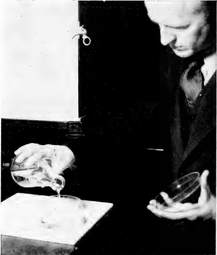
FIGURE 13.—A small amount of casting sirup is first poured into the mold and polymerized to serve as a supporting base for the specimen.
