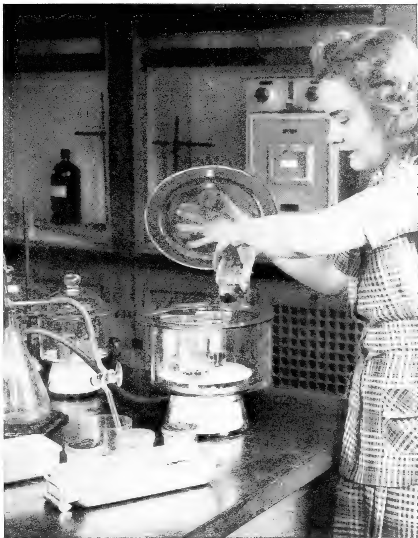
FIGURE 15.—Bubbles in the casting sirup and entrapped air in the specimens are removed after filling the molds by placing them in a vacuum desiccator. The small quantity of vapor is removed from the closed desiccator by suction.
