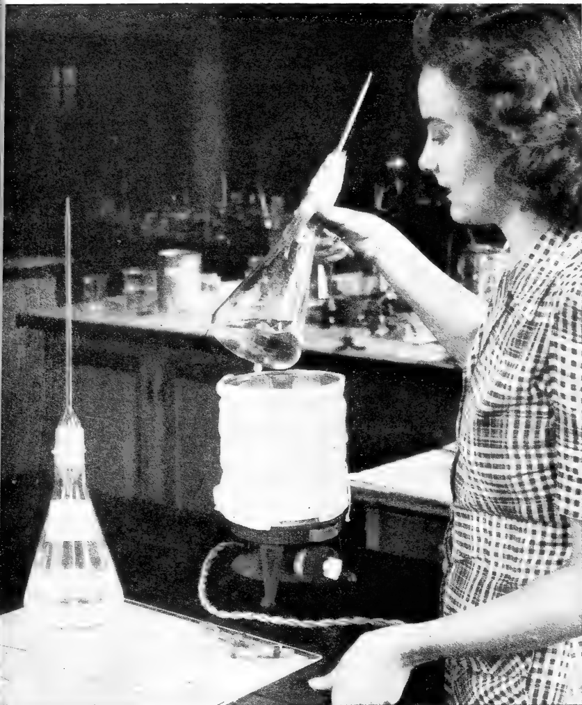
FIGURE 12.—A transfer pipette of suitable size, with the sucking end cut off and the bulb wrapped with cellophane to fit the flask's neck, provides a vented stopper which condenses the vapor and prevents its escape. Because the flask might break, it is safer to heat it under a fume hood, and to leave it there until contents are cool.
