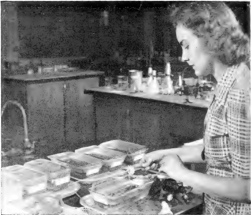
FIGURE 1.—Preliminary tests with representative color-preserving fluids may be required to determine the stabilization treatment needed for each type of plant material. Wooden or plastic forceps are used to handle the samples.
