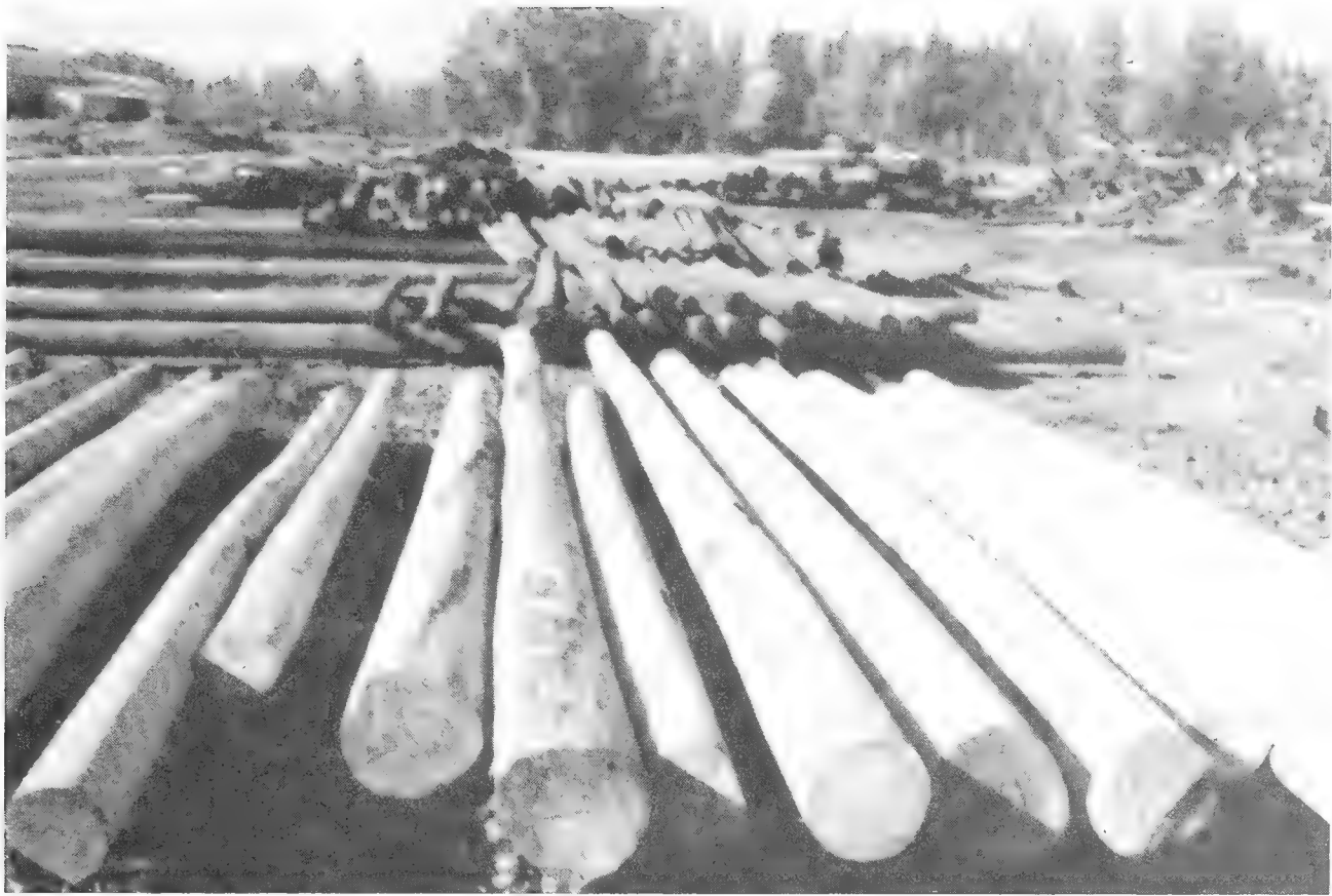
Figure 3.--A few poles spread for examination and end sampling prior to treatment by the hot and cold bath method.
