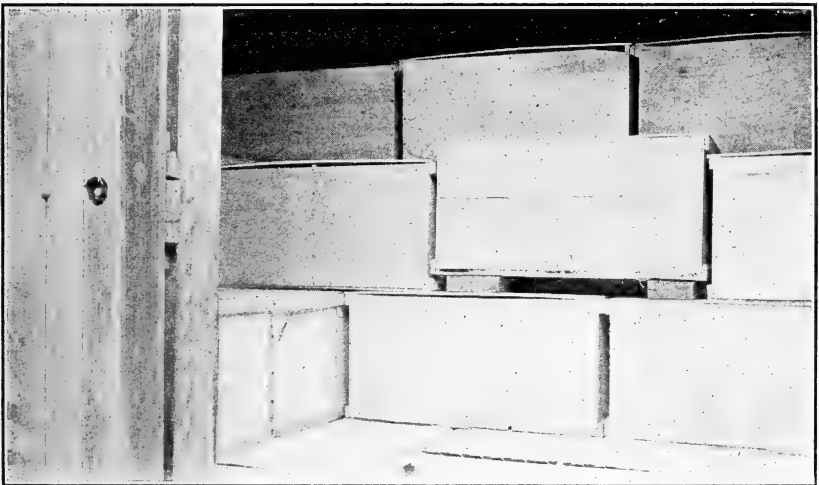
FIG. 2.—LATERAL BRACES UNDER ALTERNATE CASES, STEP-JOINT LOAD, PLACED FROM THE SIDE, SHOWING BRACES (VIEWED FROM DOOR.)
