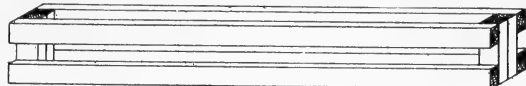
FIG. 2.—Frame placed in front of ice bunker to keep the straw buffing from blocking the cold-air exit in straw-buffed cars.
