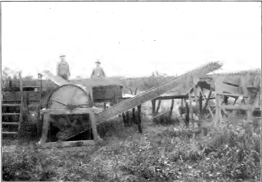
FIG. 2.—A TYPE OF PEAR CUTTER, AS SET UP AND OPERATED BY J. C. GLASS. THE PRICKLY PEAR AND A PEAR MACHINE.
