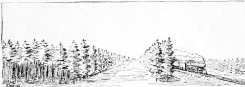
FIG. 33.—A fire line along a railroad with two cleared spaces separated by a double row of trees intended to catch the sparks.
