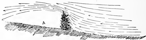
Fig. 5. Deflection of winds by a dense shelter belt.
