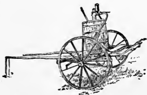
Fig. 69. Outfit for spraying strawberries and potatoes.
