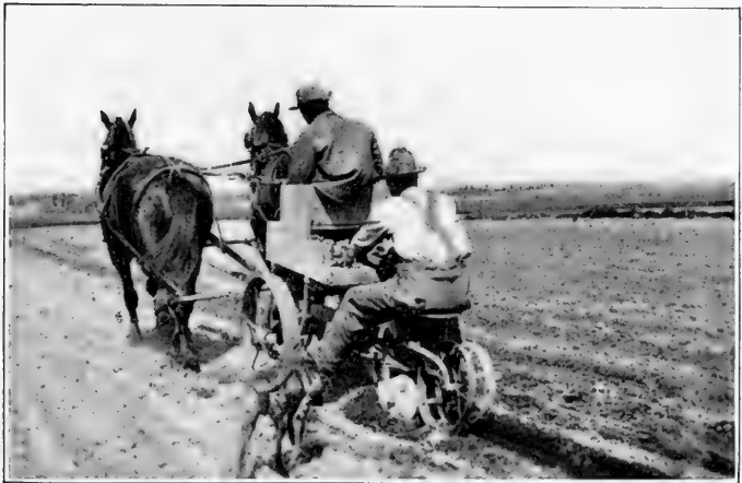
FIG. 62. — Potato planter at work: notched-wheel type.
