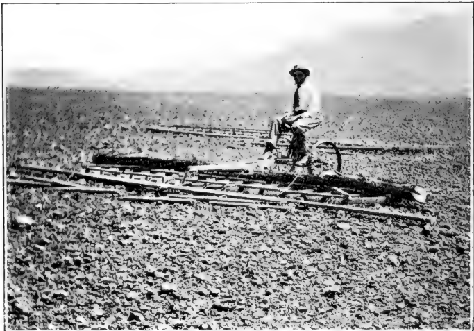
FIG. 33. — A large mulching implement used in dry-farming.
