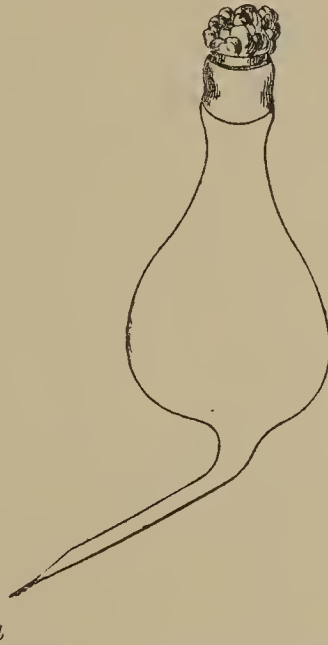
Nuttall's bulb for collecting blood-serum under antiseptic precautions.
