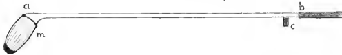
FIG. 404. Diagram of Marey's cardiac 'sound,' consisting of a long tube ab , terminating at one end in the ampulla m , which is covered with an elastic membrane. The side-piece c serves to indicate the position of the ampulla after it has been introduced into the vessels.
