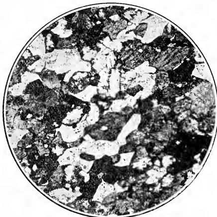
FIG. 2. Photomicrograph of diorite rock. Compare with Figs. 3, 5, and 6, which have a different mineral composition, crystalline form and structure. These differences determine the type and rate of their weathering. (Lord.)
