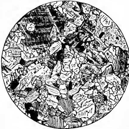
FIG. 1. Section of granite, magnified. The crystals are orthoclase, microcline, plagioclase, quartz, black mica or biotite, white mica or muscovite. (Merrill.)
