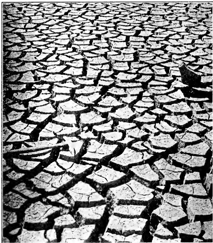
FIG. 29. Excessive checking of a heavy clay soil as a result of drying. Illustrates the process of soil granulation.
