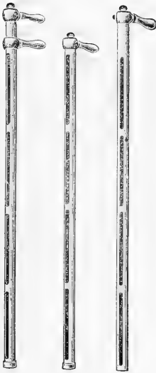
FIG. 55.—The McKay cream and milk sampler.
