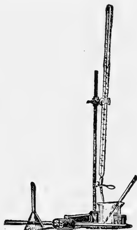
FIG. 129.—Apparatus for Mann's acid test. Instead of the burette the alkali can be kept in a large bottle, as shown in Fig. 131 and 130.
