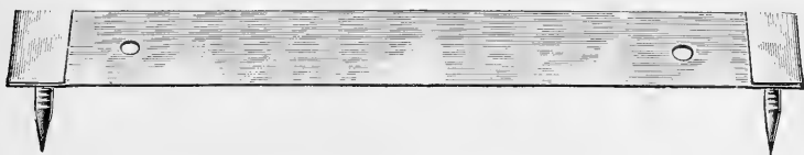
FIG. 163.—Tub-fasteners; tin and tack combined.
