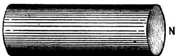
Fig. 36. Bar magnet with magnetic moment \mathfrak{M} = ml ; equivalent to solenoid in preceding figure.
