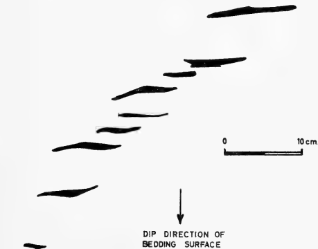
Fig. 3. Sketch from a photograph of a part of shear zone (f) showing gently deformed en-échelon veins.
