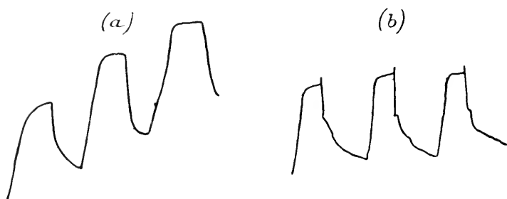
FIG. 14.—(a) Response curves of artificial retina for short periods of illumination followed by darkness. The ascending portions show the growing effect of light, the horizontal portion the balancing tetanic effect. The descending portion of the curve exhibits recovery during the absence of light. (b) Same in frog's retina (Waller).
