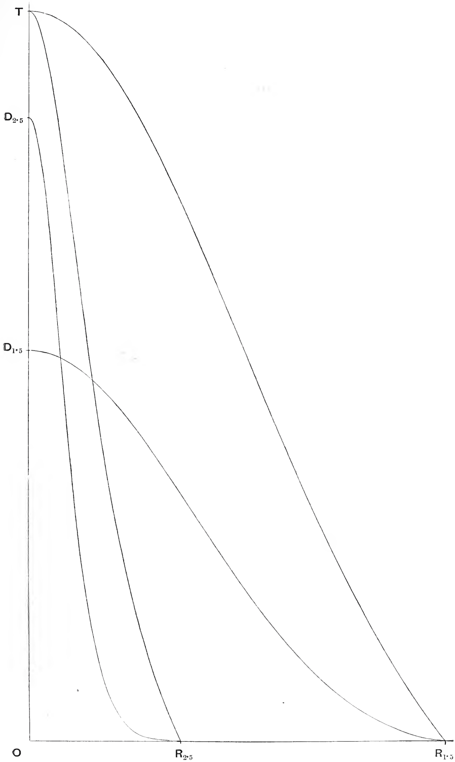
T R_{1.5} is the curve of temperature, and D_{1.5} R_{1.5} is the curve of density, for a monatomic gas ( k=1\frac{2}{3} ). T R_{2.5} , and D_{2.5} R_{2.5} are corresponding curves for a diatomic gas ( k=1.4 ).
