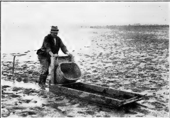
Fig. 2.—SKID OR "MUD-HORSE" USED FOR CROSSING THE SOFT OOZE TO VISIT FISHING GEAR.
