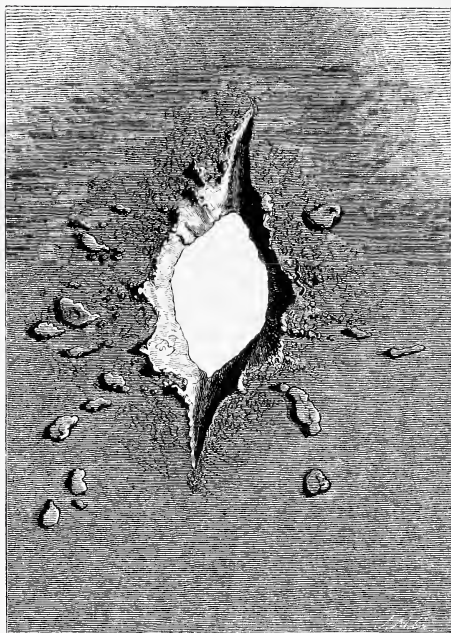
The hole at "A," as it appears on the under surface of the lead ; carefully drawn full size by Mr J. M. Corner, wood-engraver.
