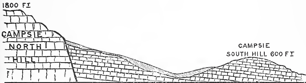
Section across Campsie Valley ; coal and limestone strata overlaid by gravel and earth.
