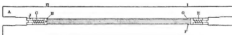
FIGURE 1. Apparatus for measuring the linear compressibility of rods. The rod to be measured is indicated by the shading. The stop D is held permanently against the shoulder B by the spring C, which is kept compressed by the pump connections, not shown. The brass ring F is kept in contact with the shoulder G during increase of pressure by the spring E, which pushes the shortening rod through the ring F, so as always to be in contact with the stop D. When pressure is released the ring comes back with the rod and the displacement is measured. The rod is removed through the end E to make these measurements; the connections at A to the pressure pump are not disturbed during the measurements. The elongation of the cylinder is measured externally at the scratches H and I.
