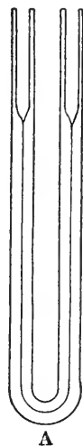
FIGURE 5. Original and final form of the receptacle for holding the mercury whose resistance is to be measured. If the glass is too thick, it invariably breaks under pressure at the bend A.
