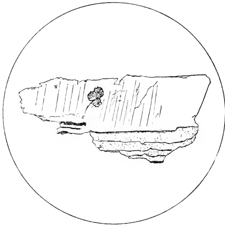
Fig. 21. Twinned crystal of labradorite, showing cleavage. \times 60 .
