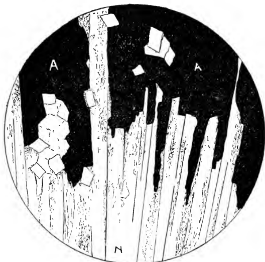
Fig. 25. Natrolite (N) and analcite (A) between crossed nicols. \times 30 .
