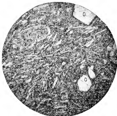
Fig. 23. Section of the basaltic facies (specimen 38), showing basaltic and flow structure. (O), olivine; (O'), olivine weathering to iddingsite; (F), feldspar crystal with etched edges; (A), augite. \times 20 . Photograph by Ralph Arnold.
