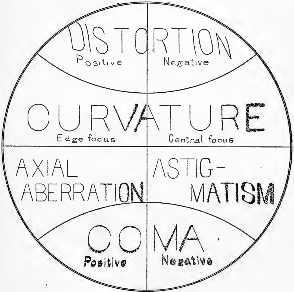
Fig. 1. Chart illustrating the appearance under the microscope of the five spherical aberrations.
