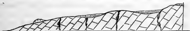
Fig. 6.—Section showing modes of occurrence of Fissures and Faults in the Carboniferous Limestone, with patches of Dol. Conglomerate and New Red lying in hollows, &c.
