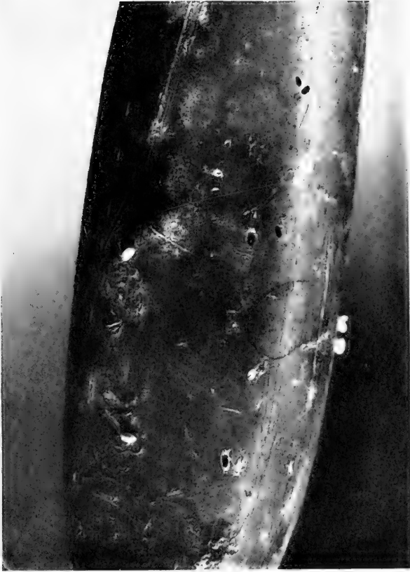
Section of lead telephone cable showing eggs of M. stigma and holes made by larvae.
