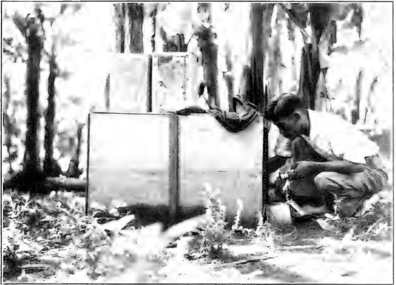
Figure 5. -New style trap lined with earth showing method of removing mosquitoes. Note drip cans on top.
