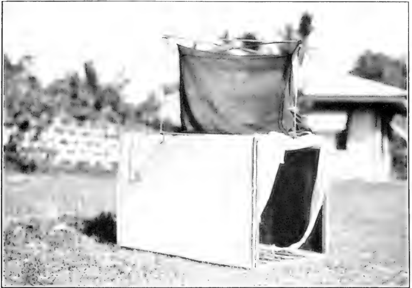
Figure 1. —Unlined (old style) mosquito trap. Showing inside catching chamber removed.
