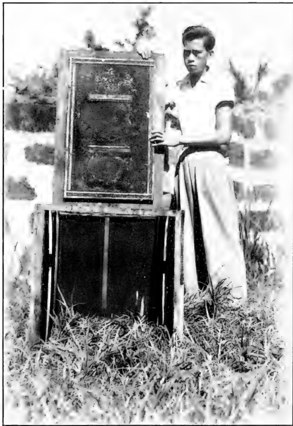
Figure 3. —New style trap lined with earth. Front open. Top removed for photograph.
