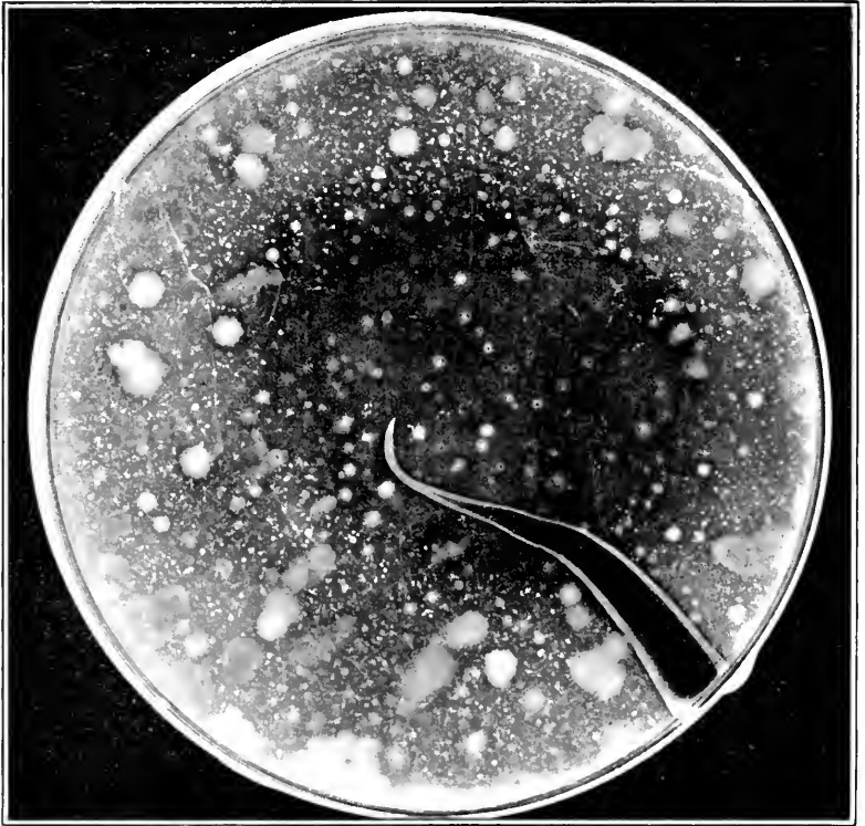
Agar Plate, showing colonies of bacteria in 1/500 centimeter of sewage as entering Septic Tank.
