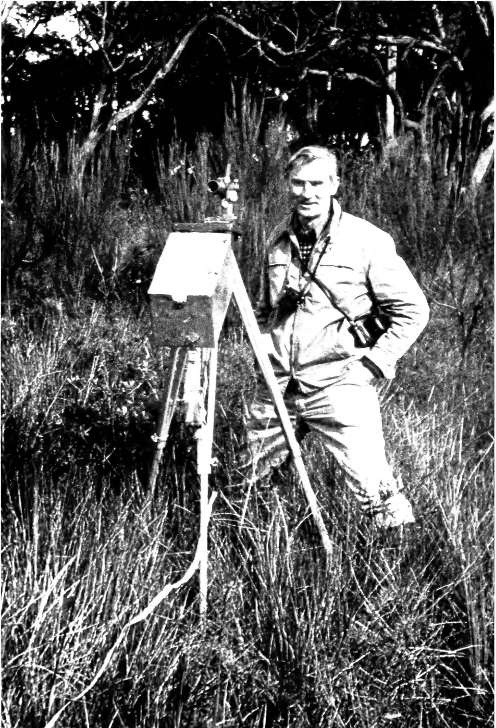
Peter Myerscough surveying an upland swamp with an alidade, near Darkes Forest, N.S.W.
