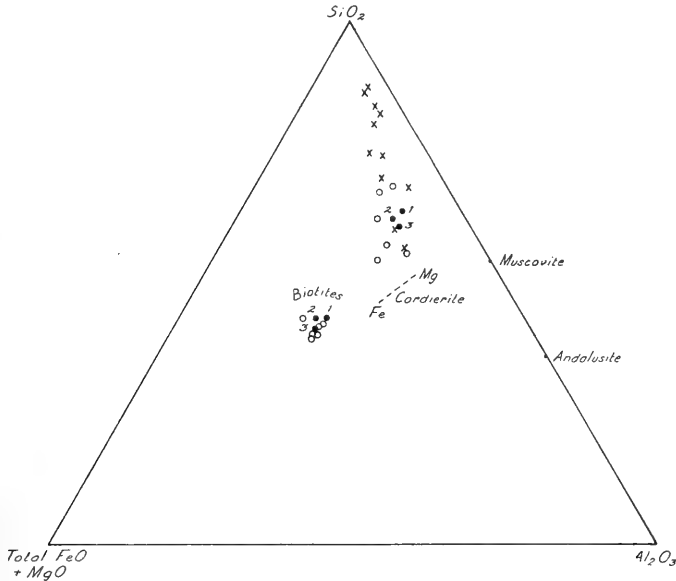
Figure 3. SiO_2 - Al_2O_3 - \text{total FeO} + MgO diagram showing the relation between biotites and their host rocks. The spots refer to the analyses in this paper, the crosses represent other analysed metasediments from the Wantabadgery-Adelong-Tumbarumba district (Vallance, 1953a). Biotites and host rocks from Deeside (Snelling, 1957) are indicated by open circles. Important phases which may co-exist with biotite in the present area are plotted on the diagram.
