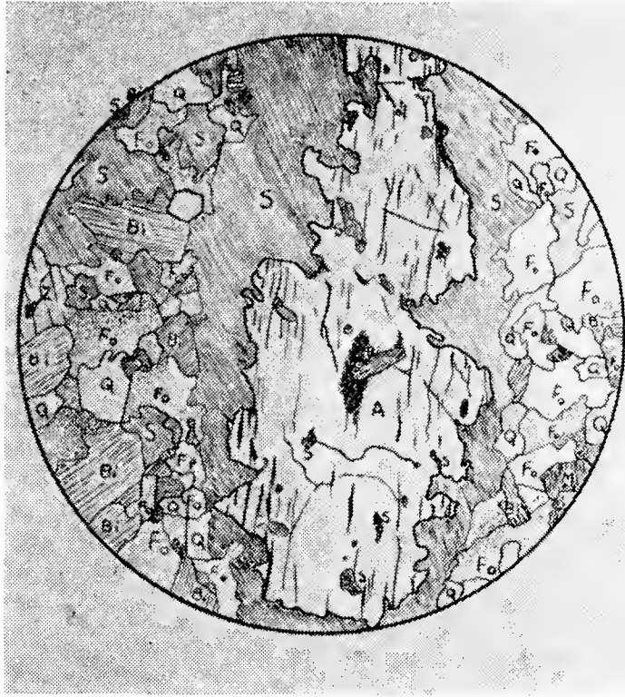
Fig. 4. Andalusite (A) being altered to sericite (S). Quartz (Q), orthoclase (Fo), biotite (Bi), muscovite (M). X20.
