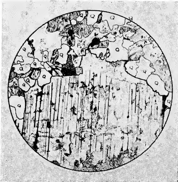
Fig. 3. Albite porphyroblast (Fp) growing in a matrix of quartz (Q), orthoclase (Fo) and biotite (Bi), X20.
