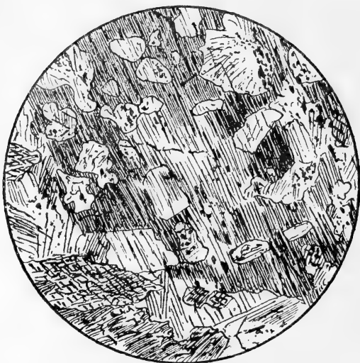
FIG. 1.—Section of amphibolite of Cor, Co. Donegal, showing traces of ophitic structure. The pale spaces are occupied by actinolite, associated with magnetite; the fibres of actinolite are sometimes in continuity with those of the darker hornblende round it. \times 9 .
