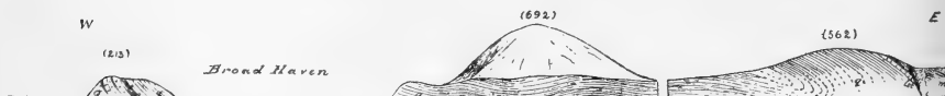
FIG. 3.—General Section from Erris Head hill (213) across Broad Haven eastward to Glencalry hill (562) showing gneiss (G), quartzite (q), limestone (lst), and mica-schist (m), faulted beyond overfold.
