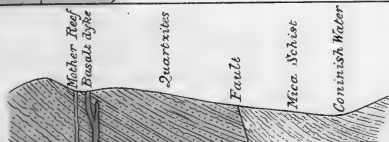
Fig. 1. SECTION ALONG LINE A. B.
