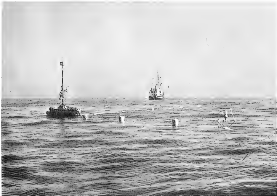
Figure 2. Buoy with gyro-stabilized mast carrying sensors for recording the fluctuations in horizontal and vertical wind components and in air temperature. In the foreground: small buoy for recording the wind speed close to the sea surface. In the background: research vessel "Hermann Wattenberg" of the Oceanographic Institute at Kiel University connected by floating cable with the buoy. (By courtesy of Dr. K. Brocks.)
