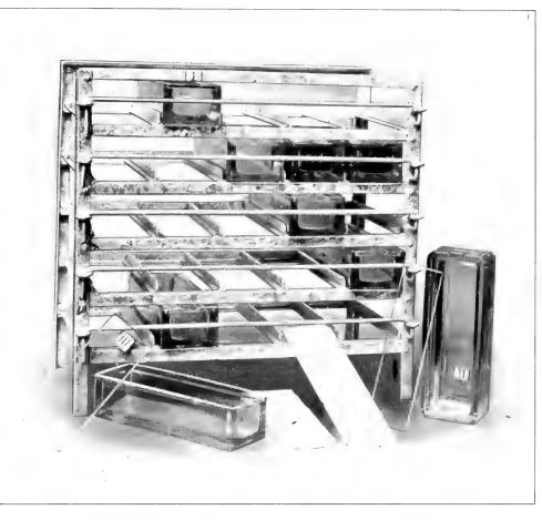
FIG. I. A view of the "angle iron" frame holding seven glass trays. Two additional trays in different positions, with their glass lids leaning against them, are shown. The white objects in the foreground are paraffined muslin strips, which are used with the glass lids to effect air tight closure of the trays.
