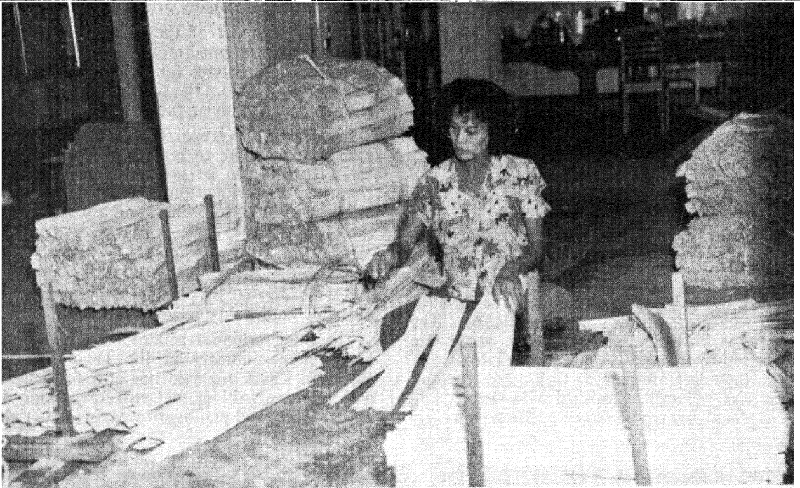
Fig. 2.—Grading of the bi-lobed slips.
