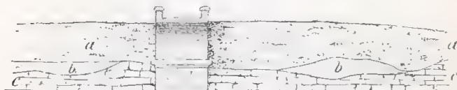
Fig 2. Section of Limestone and Middle Marls.
