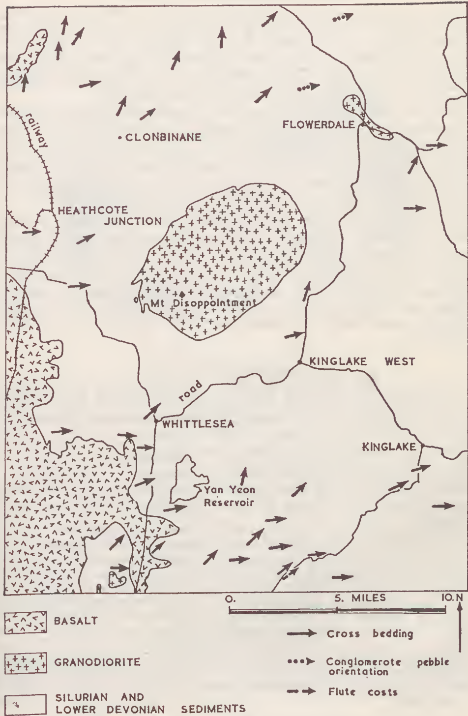
FIG. 5—Palaeocurrent directions within the area investigated. Vector mean of 77 cross-bedding measurements strikes 50°; vector magnitude 70%.
