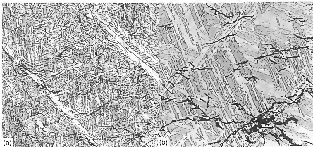
Fig. 10. Typical structures in Willow Grove meteorite. The main feature is lath martensite, forming the plate-like texture, crossed by a network of microcracks [field of view is 1.6 mm across in (a), 0.3 mm across in (b)].
