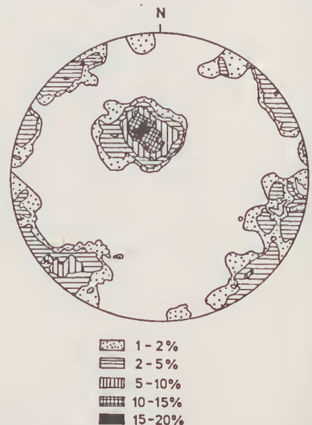
FIG. 6—Equal area projection of planar discontinuities (bedding and jointing) at Windy Point. 102 points.
