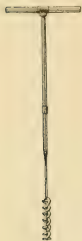
FIG. 183.—A soil auger made by welding a \frac{3}{8} -inch gas pipe to a 1\frac{1}{4} -inch wood auger. An excellent tool in its proper use in estimating the value of land.
